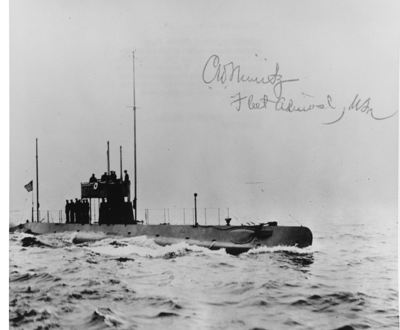
Early submarine with wireless mast deployed, as signed by Fleet Admiral Chester W. Nimitz. (U.S. Navy photo)
