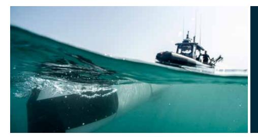
A Mk-18 Mod 2 UUV with the ATLAS forward looking sonar module attached begins its dive for a mine hunting mission.
