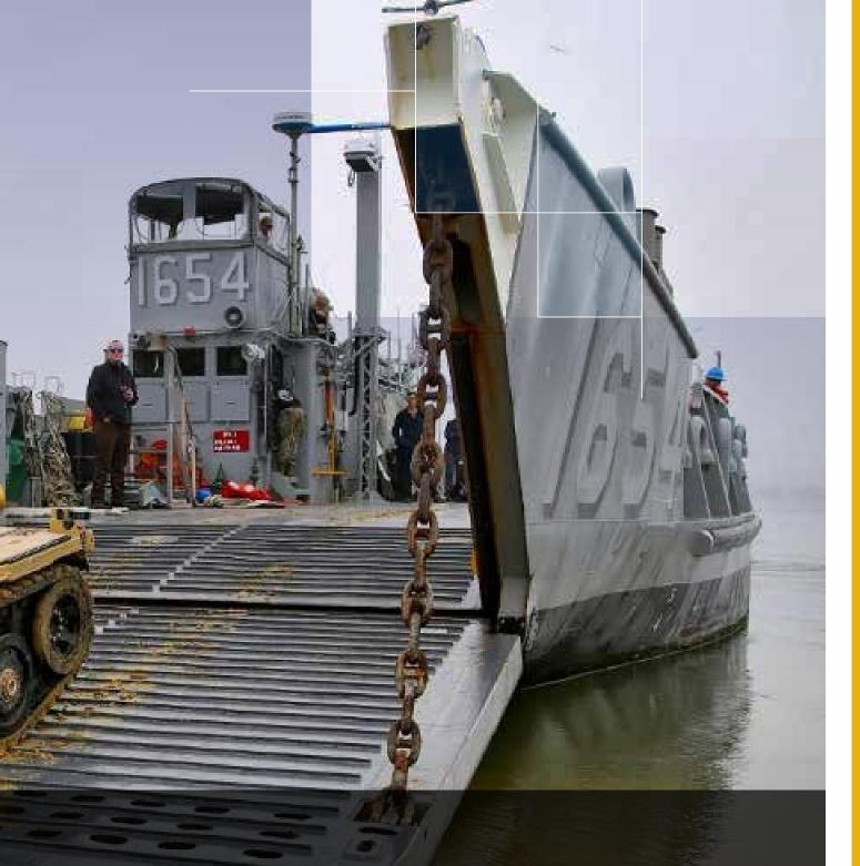
A Marine Corps Warfighting Laboratory Robotic Combat Vehicle-Light (RCV-L) autonomously departing an Assault Craft Unit-2 Autonomous Littoral Connector (ALC), a legacy Navy landing craft outfitted with sensors and software giving the craft both remote-control and full autonomous capabilities.
