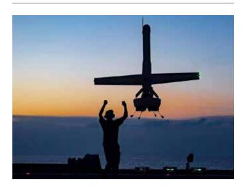
A VBAT vertical take-off and landing (VTOL) unmanned aerial system (UAS) prepares to land on the flight deck of a naval ship.
