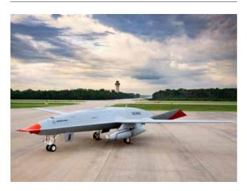
MQ-25 T1 with Aerial Refueling Store under left wing, on the ramp.
