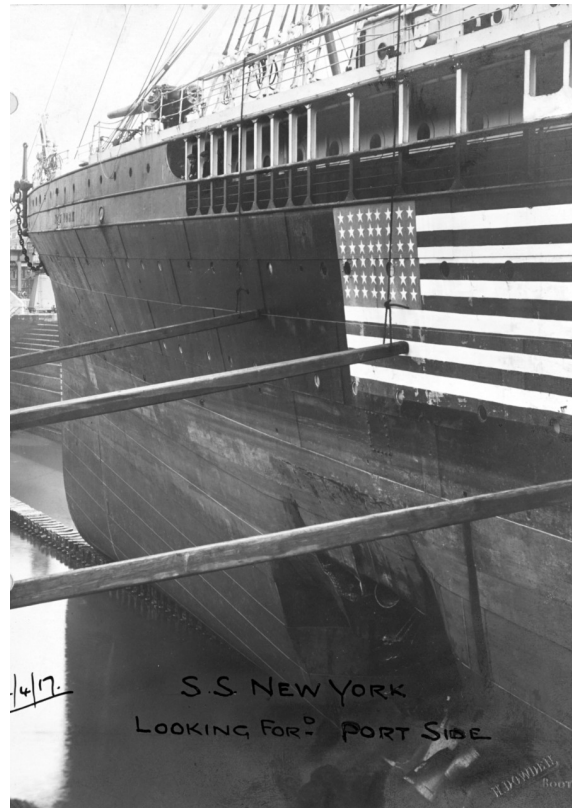
SS New York damaged by German mine in the approaches to Liverpool with Sims on board in April of 1917. (U.S. Navy)
